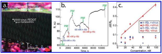
FIGURE 4. (a) Optical micrograph of a virus-PEDOT nanowire array device. (b) Raw biosensing data, taken in real-time with the indicated injections of negative antibody (n-Ab, blue arrows), positive antibody (p-Ab, red arrows), or washes with PBF buffer (green arrows). (c) A compilation of all real-time biosensing data, depicted as a calibration curve, in which the resistance change upon injection is plotted versus analyte concentration.
