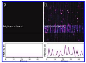
FIGURE 3. (a) A fluorescence microscopy image of PEDOT nanowires after incubation with anti-M13 antibody conjugated to fluorescein. As expected, minimal fluorescence intensity is observed (lower). (b) A fluorescence microscopy image of virus-PEDOT nanowires following incubation with anti-M13 antibody conjugated to fluorescein shows localization of the viruses to the nanowires. Image J analysis quantifies the increased fluorescence intensity at the wires (lower).
