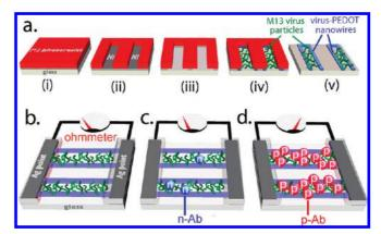
FIGURE 1. (a) Schematic diagram of the LPNE process for the synthesis of virus-PEDOT nanowires. (b) The resultant virus-nanowire device used for resistance-based measurements. (c) Schematic, indicating little to no change in resistance after treatment with a nonbinding negative control antibody (n-Ab, blue circles). (d) Depiction of the substantial change in resistance due to the presence of virus-binding positive antibody (p-Ab, red circles).
