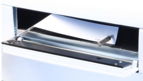
Figure 3. Transport lock bar with warning tag
