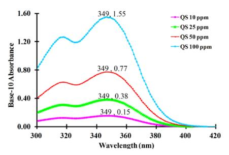
(b) Calibration of the measured base-10 absorbance vs. QS mass concentration in ppm. The QS concentration used in the fluorescence measurements was 0.1 ppm; the corresponding absorption coefficient calculated from the linear fit is 0.00155 cm<sup>-1</sup> at the peak of the QS absorption spectrum (349 nm).
