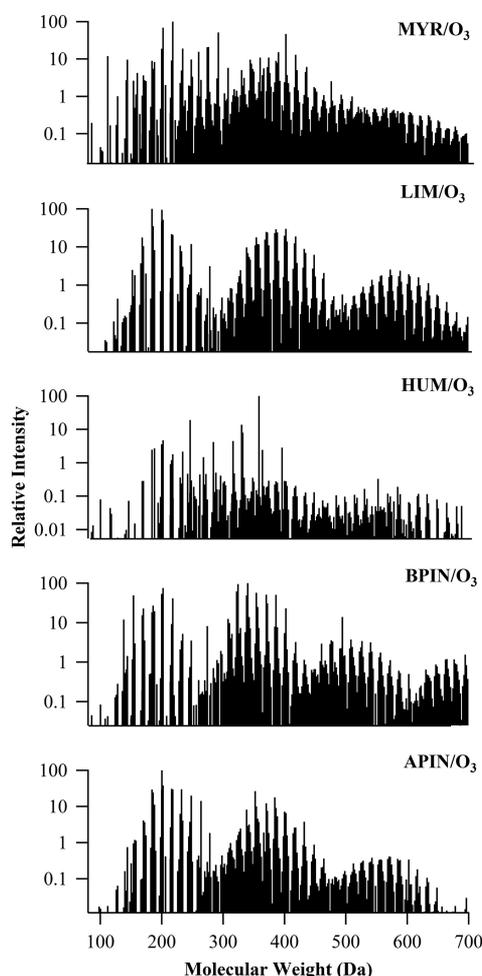
**Figure 2.** Reconstructed mass spectra for all VOC/O<sub>3</sub> SOA samples (before photolysis) recorded in this work. The *x*-axis corresponds to the molecular weight of the neutral SOA compounds. The *y*-axis is on a log scale to make the weaker peaks of oligomeric compounds easier to see.
