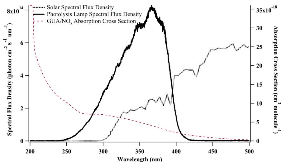
**Figure 1.** Spectral flux density in the photolysis cuvette compared to the solar spectral flux density at SZA = 0. The right axis shows the effective absorption cross-sections of GUA/NO<sub>x</sub> calculated from eq 1.
