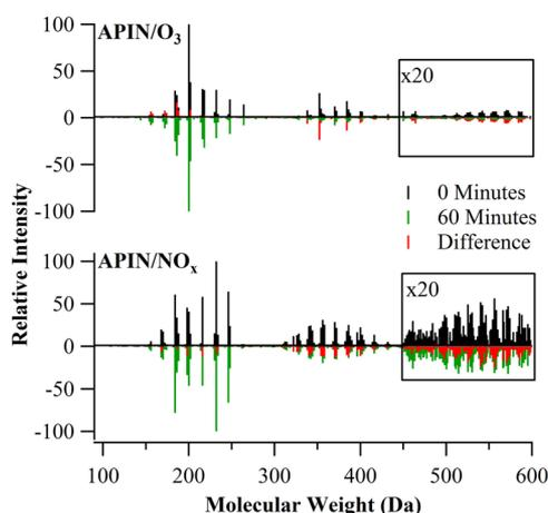
**Figure 4.** Mass spectra of APIN/O<sub>3</sub> and APIN/NO<sub>x</sub> SOA solutions before (black) and after (green) 1 h of photolysis. The mass spectra after photolysis are inverted for clarity. The difference (red, after – before) is representative of the change that occurred during the photolysis time.
