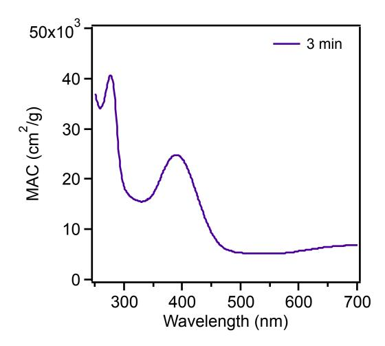
**Figure S9:** Mass-normalized absorption coefficient (MAC) plot for the reaction of 1 mM catechol with  $FeCl_3$  after 3 min dark reaction at pH 3 (unfiltered solution). The final reaction mixture contain 1:2 molar ratio catechol:Fe. MAC was calculated from Eq. (1) and it was not corrected for the contribution from scattering by particles in solution.
