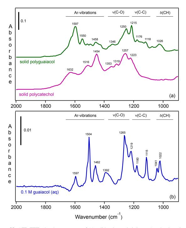
**Figure S8:** ATR-FTIR absorbance spectra of (a) solid polycatechol (bottom) and polyguaiacol (top) deposited on a ZnSe ATR crystal from a water/ethanol slurry followed by drying overnight, and (b) 0.1 M aqueous solution, and Similar spectra of catechol monomers were reported earlier.<sup>4</sup>
