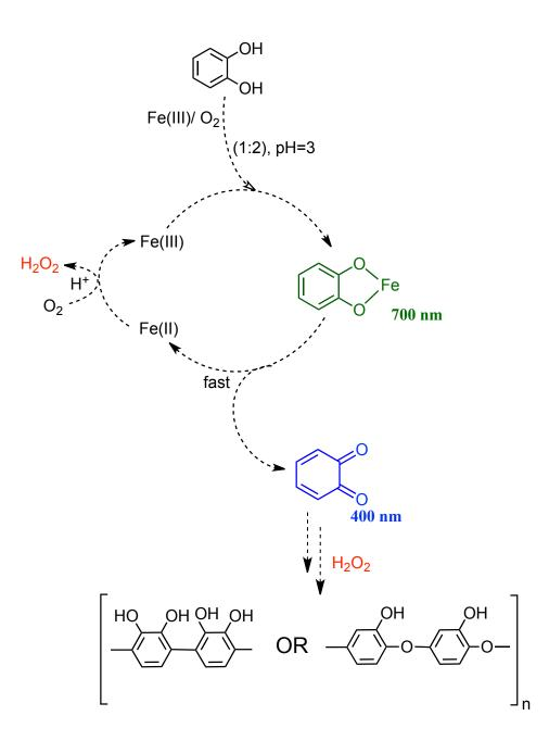
Scheme S2: Suggested mechanism for catechol oxidation and polycatechol formation in the presence of excess Fe(III) in the dark under acidic conditions.
