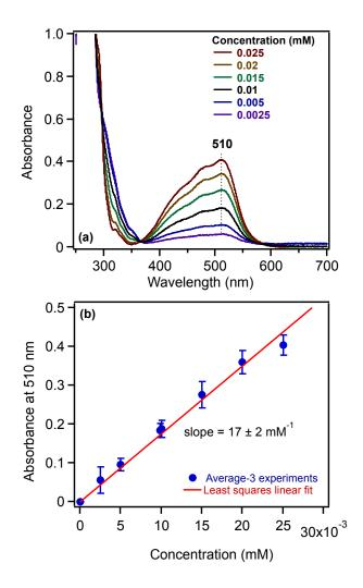
**Figure S1:** (a) Representative UV-vis absorbance spectra of the complexes between standard solutions of  $(NH_4)_2Fe(SO_4)_2\bullet 6H_2O$  and 1,10-phenanthroline. (b) Calibration curve constructed from the absorbance at 510 nm from spectra shown in panel (a).
