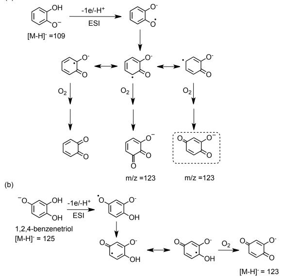
Scheme S3: Suggested mechanism for the oxidation of (a) catechol and (b) 1,2,4-benzenetriol induced in the ESI chamber by  $O_2(aq)$  explaining the origin of the m/z 123 with the same fragmentation pattern for both chemicals.
