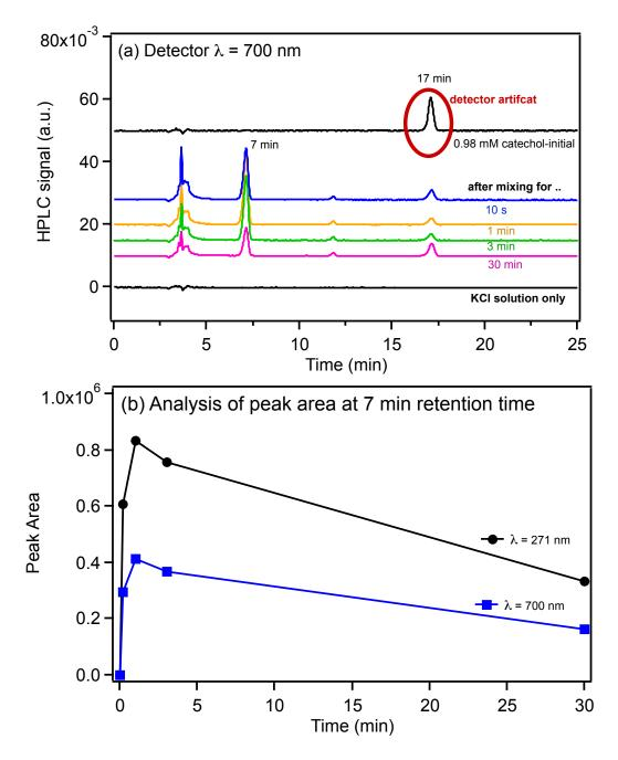
**Figure S4:** (a) HPLC chromatograms collected for initial catechol solutions (0.98 mM) and after reaction with FeCl<sub>3</sub> at pH 3 as a function of reaction time with a final molar ratio of 1:2, and (b) kinetic curves for the product peak at 7 min as a function of detector wavelength. The phrase "detector artifcat" refers to the signal at 700 nm for the 17 min peak that does not originate from the catechol standard solution in the absence of iron.
