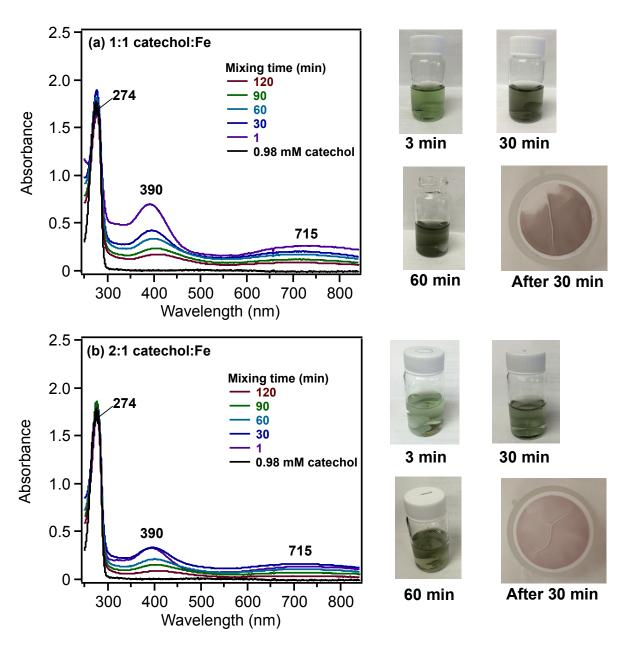
**Figure S2:** UV-vis spectra of unfiltered solutions after dark reaction and filtration of catechol (0.98 mM) with  $\text{FeCl}_3$  at pH 3 at different ratios a function of time. Digital images of the corresponding unfiltered solutions and particles on filter after 30 min are shown on the right.
