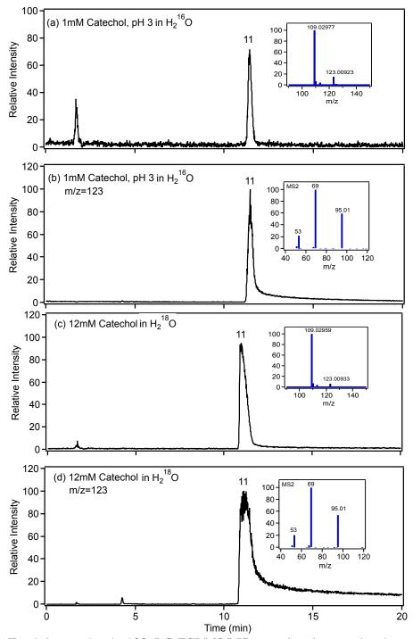
**Figure S5:** Total ion and m/z 123 LC-ESI-MS/MS negative ion mode chromatograms for catechol standard solutions under acidic conditions in normal water (H<sub>2</sub><sup>16</sup>O, (a)-(b)) and in water-<sup>18</sup>O (H<sub>2</sub><sup>18</sup>O, (c)-(d)). The insets in (a) and (c) show the mass spectra for the major peaks, and those in (b) and (d) show the MS/MS spectra for the m/z 123 ion.
