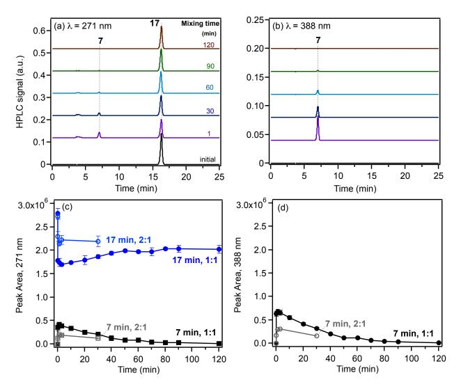
**Figure S3:** (a) and (b) HPLC chromatograms collected for initial catechol solutions (0.98 mM) and after reaction with  $FeCl_3$  at pH 3 as a function of reaction time with a final molar ratio of 1:1. (c) and (d) The resultant kinetic curves from the integrated areas of the peaks at 7 and 17 min for solution mixtures containing 1:1 and 2:1 molar ratio of catechol:Fe.
