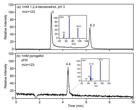
**Figure S6:** Chromatograms for m/z 123 of reference compounds 1,2,4-benzentriol and pyrogallol under acidic conditions in normal water (H<sub>2</sub><sup>16</sup>O). The insets show the MS/MS spectra for the m/z 123 fragment.
