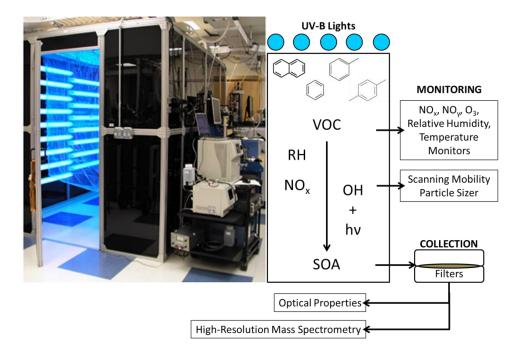
Figure 1.1: Photo and diagram of chamber setup
