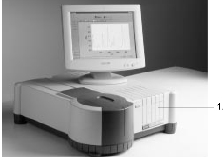
The snap-out panel (1) on the front of the Cary 50
