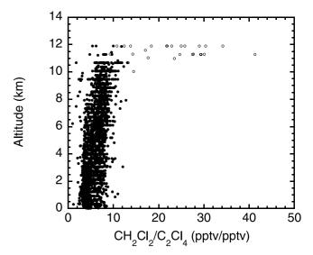
Figure 1. Altitude profile of CH<sub>2</sub>Cl<sub>2</sub>/C<sub>2</sub>Cl<sub>4</sub> for air samples that passed the data editing procedures outlined in the text. Open circles are from the four air parcels that showed depleted C<sub>2</sub>Cl<sub>4</sub>.
