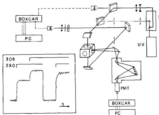
Fig. 2. Experimental diagram showing geometry used for small-signal gain measurements and pump-dump experiments. Inset shows boxcar-averaged intensity levels obtained during gain measurement (see text for explanation).
