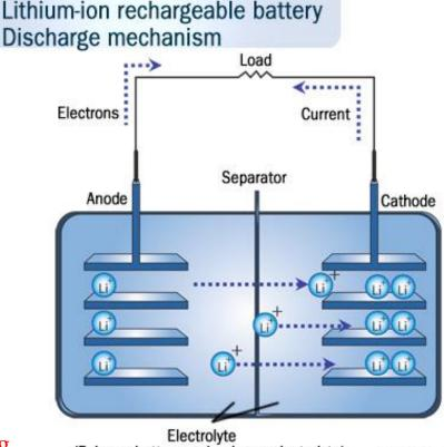
(Polymer battery: gel polymer electrolyte)
