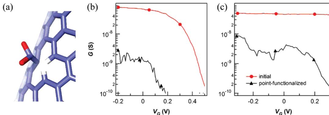
**Figure 1.** (a) Model for a carboxylate point defect electrochemically introduced into a SWCNT sidewall. (b,c)  $G(V_g)$  characteristics for devices composed of one semiconducting SWCNT (b) and one metallic SWCNT (c).  $G(V_g)$  is shown before (red) and after (black) point-functionalization of each device. The decrease in conductance and change in  $V_g$  sensitivity are attributed to the incorporation of a carboxylate.
