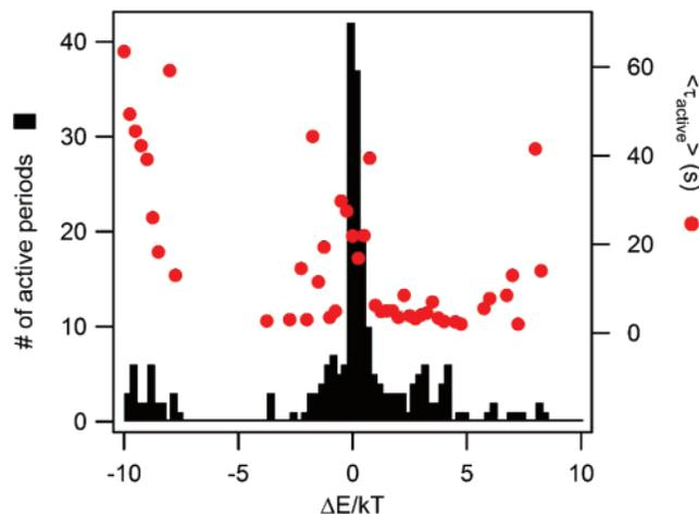
**Figure 5.** Histogram of  $\Delta E$  values shows the preponderance of active events have symmetric fluctuators with  $\Delta E \sim 0$  (black). Fluctuators with  $\Delta E$  of a few  $k_B T$  tend to have relatively short lifetimes (red), except for a population of unusually long-lived fluctuators with  $\Delta E < -7 k_B T$ .
