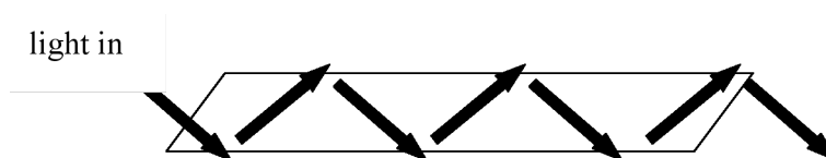
Figure 4: Schematic diagram of multiple reflections inside a multipass ATR accessory
