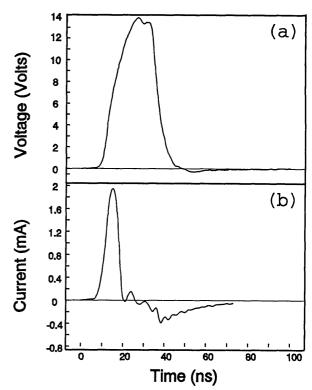
Fig. 9. Waveforms measured with a C30902S and the active quench circuit: (a) Variation of voltage across the APD, (b) current flowing through the diode.
