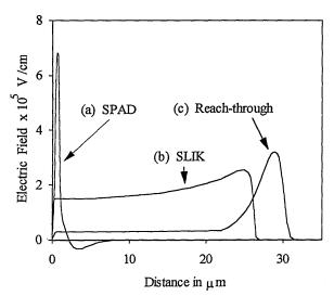
Fig. 1. Field profile of three APD structures that can be used for photon counting: (a) the SPAD (a single-photon APD) developed by Cova *et al.*, (b) reach-through structure; (c) Slik design.
