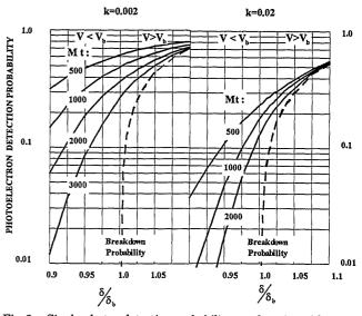
Fig. 3. Single-photon detection probability as a function of discriminator threshold setting Mt (in electrons) for two types of APD.
