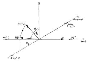
FIG. 2. Representation of "radiation damping" with the complex Maxwell's equations represented on the I-II plane by the hollow arrows.  $\mathbf{R} = \Sigma i \mathbf{r}^i$ ,  $\alpha = f V^{-i} \mu_{\alpha b}$ , P = total polarization (or magnetization).
