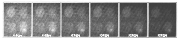
Figure 7. "Melting movie" showing changes in the in situ SPR image of the hybridized surface from Figure 6b as temperature is gradually raised. The cell temperatures at which the images were acquired are listed in the figure.
