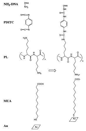
Figure 1. Schematic of method used for coupling 5'-amineterminated oligonucleotide probes to a gold surface.
