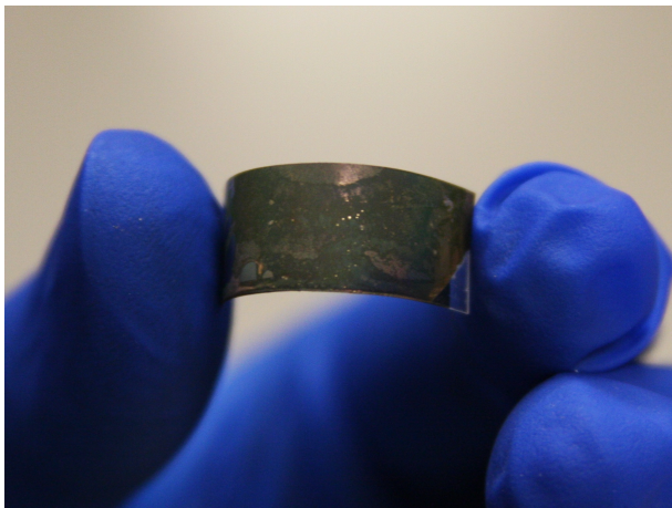
Gold-coated plastic nanocone array
